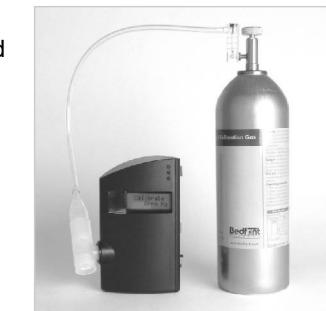
Open the fine control valve and allow the gas to flow at 0.5 litres/minute. To maintain this, adjust the flow so the ball in the Flow Indicator remains at the lower line (see diagram opposite).
