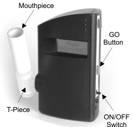
2. Unit will automatically enter a Zeroing mode, taking up to 2 minutes.
