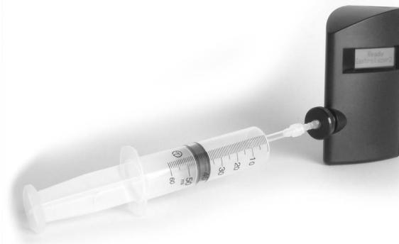
Connect the syringe to the sampling plug using the plastic tubing (see photograph opposite). Start the test in the normal way and when the display shows:
