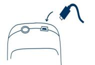
Place one end of the connection lead into the USB socket on the top of the Gastro<sup>+™</sup> Gastrolyzer<sup>®</sup> product.
