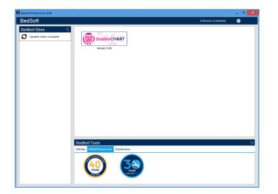
Once Bedsoft has been downloaded and user accounts enable/disabled, GastroCHART<sup>™</sup> can be downloaded and installed from the left hand side of the screen, under the Bedfont<sup>®</sup> Store heading. Once GastroCHART<sup>™</sup> installation is complete, the software tab will move into the centre of the screen, as shown.
