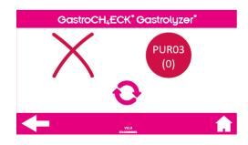
CH<sub>4</sub> sensor sync error: Press the retry button. If the error occurs more than 3 times, please restart the unit. If failure persists contact Bedfont® or their distributor for support.
