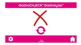
Calibration failed: Check calibration gas tubing is connected to the breath sampling port.
