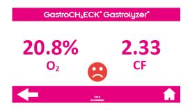
This will show the  $O_2$  concentration in % and the correction factor applied to the reading if it was required. A visual indicator will help to interpret the result:
