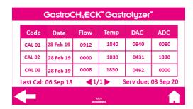
**NOTE:** Calibration errors will only appear in the log and not as a separate warning. The possible errors are:
