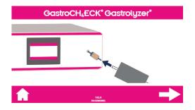
The device will then illustrate to attach the breath bag. Carefully remove the blue plug on one end only and attach the bag to the moisture filter, then open the clamp on that end only to preserve the sample.
