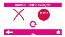
$O_2$  sensor zero failure: Reattempt breath test or bag test. If failure persists contact Bedfont® or their distributor for support.
