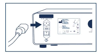
3. Switch the monitor on using the ON/OFF switch at the back of the unit. The screen will light up and if any warning screens are displayed, these should be checked in the Troubleshooting section of the manual.
