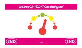
An on-screen dial will help to guide the exhalation rate; keep the arrow pointing in the green section of this indicator throughout the test.
