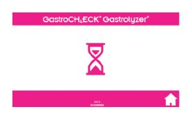
A timer will be shown onscreen whilst the sensors are zeroing. This may take up to 75 seconds if a test has just been carried out.
