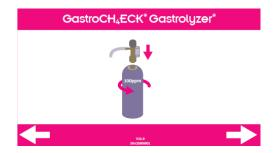
Screw the gas canister into the regulator.
