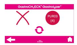
CH<sub>4</sub> sensor failure: Press the retry button. If the error occurs more than 3 times, please restart the unit. If failure persists contact Bedfont® or their distributor for support.
