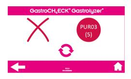
CH<sub>4</sub> sensor reading error: Verify that no gas is flowing through the device. If gas was being used, please wait 5 minutes before attempting a new test and then press the retry button. If the error occurs more than 3 times, please restart the unit. If failure persists contact Bedfont® or their distributor for support.
