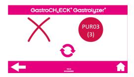
CH<sub>4</sub> sensor error: Check that the ambient temperature is within range and that the unit is plugged correctly. Then press the retry button. If the error occurs more than 3 times, please restart the unit. If failure persists contact Bedfont® or their distributor for support.
