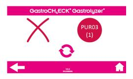
CH<sub>4</sub> sensor connectivity error: Press the retry button. If the error occurs more than 3 times, please restart the unit. If failure persists contact Bedfont® or their distributor for support.
