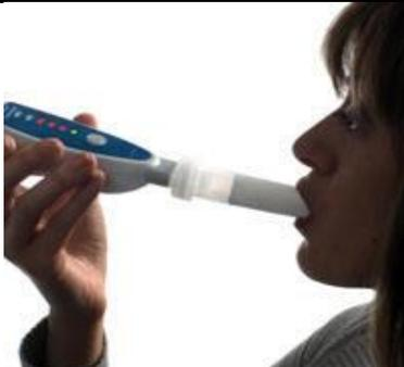
1. Insert a D-piece into the COmpact™ and fit a new cardboard mouthpiece over the D-piece.
