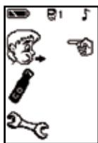
Press and hold the button for three seconds until the display becomes active. Release the button. After a 10-second warm-up period, during which a start-up screen is displayed, the main menu will appear.
